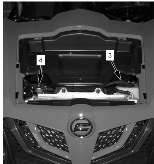
3. Reservoir Tank Cover
