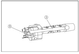
A. Clutch Lever B. Clutch Switch
