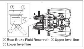
If the fluid level in either reservoir is lower than the lower level line, check for fluid leaks in the brake lines, and fill the reservoir to the upper level line. Inside the front brake fluid reservoir is a stepped line showing the upper level line.
