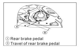
• If it does not, adjust the rear brake light switch.
