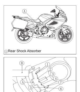
(A) Spring Preload Adjuster (B) Wrench
